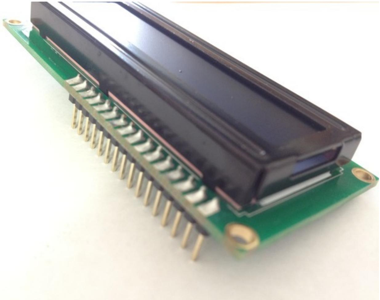
Whenever you come across a LCD that looks like it has 16 connectors it is most likely using a HD44780 controller. These devices provide the same pinouts making them relatively easy to work with. The LCD uses a parallel interface meaning that we will need many pins from our raspberry pi to control it. In this tutorial we will use 4 data pins (4-bit mode) and two control pins.
